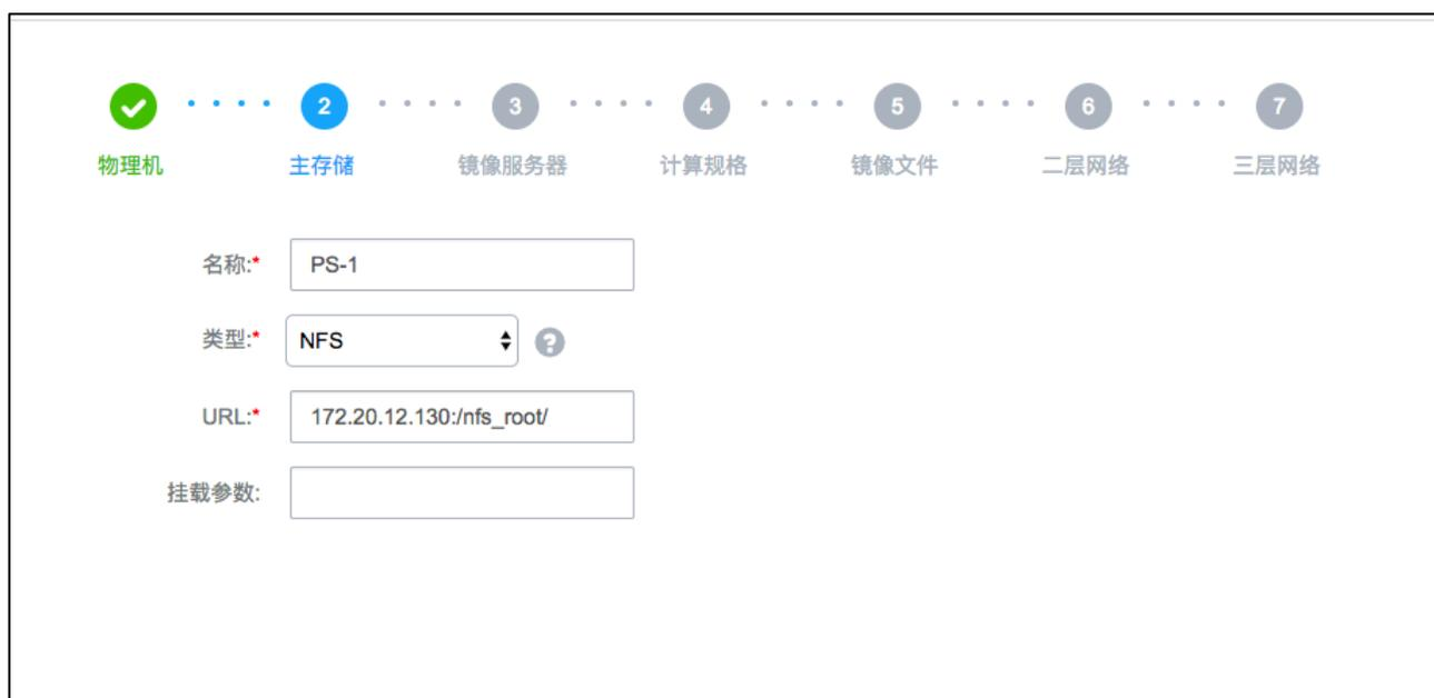
The screenshot shows the ZStack initialization wizard at step 2, '主存储' (Main Storage). The progress bar at the top indicates that '物理机' (Physical Machine) is completed (green checkmark) and '主存储' is the current step (blue circle). Other steps include '镜像服务器' (Image Server), '计算规格' (Compute Profile), '镜像文件' (Image File), '二层网络' (Layer 2 Network), and '三层网络' (Layer 3 Network). The form fields are as follows:
