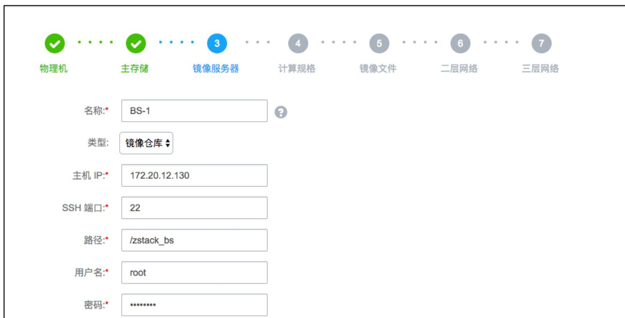
The screenshot shows the ZStack initialization wizard at step 3, '镜像服务器' (Image Server). The progress bar indicates that '物理机' and '主存储' are completed (green checkmarks), and '镜像服务器' is the current step (blue circle). The form fields are as follows:
